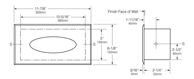
Rough Wall Opening 10-3/4" (275mm) wide 5-1/4" (135mm) high 2-3/8" (65mm) minimum recessed depth
