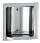
Stainless steel recessed shells are stamped from 22-gauge (0.8mm) corrosion-resistant type 304 stainless steel. Permanent soap holder is of type 304 polished stainless steel.
